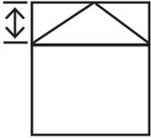
Transom location from top frame to centre of transom. Does not include frame packers and joining strips.
