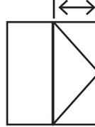
Mullion location from edge of frame to centre of mullion. Does not include frame packers and joining strips.
